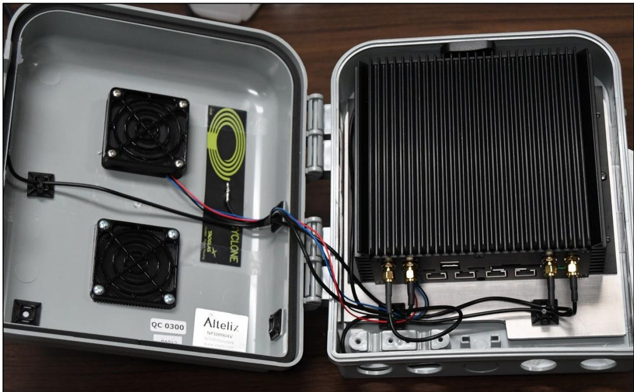
Figure 1. Master Edge Enclosure: Antennas (Left) and Box (Right)
