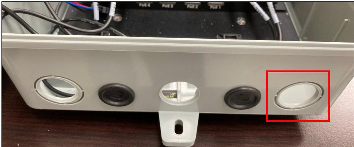
*Figure 3: Grommet Location on Enclosure*
