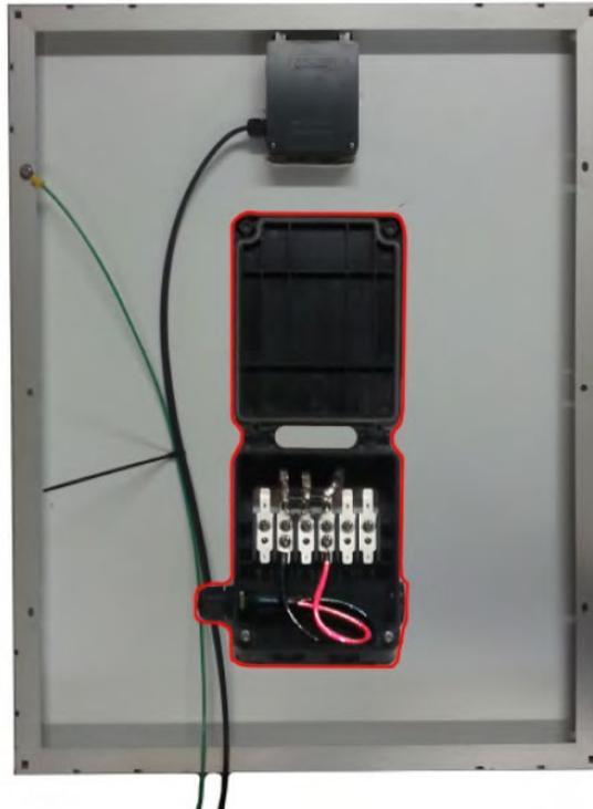
1. Route the output conductors from the solar (PV) panel to the enclosure. Secure the conductors to the panel frame or the mounting surface using wire ties or other restraining hardware (not provided). Install the cord grip fitting to the rear of the enclosure using the ½ inch knock out provided.
