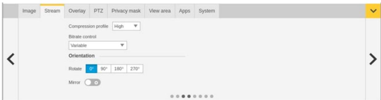
Figure 7. H.264 and Orientation Stream Settings
